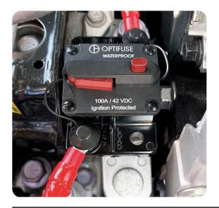
Circuit Breakers differ from fuses because they can be repeatedly tripped and reset in the event of overcurrents. They do not need to be replaced after each use like most fuses do.
