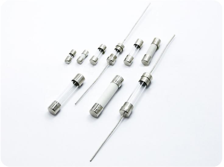
Same as for the other fuses, in order to select the proper tube fuse three electrical ratings need to be considered: nominal current, voltage, and interrupting rating. Additionally, in applications in which the fuse must sustain large current pulses of a short duration, the nominal melting I2t should be analyzed too.
