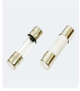
Tube fuses are available in glass or ceramic. The physical properties of the ceramic material make the ceramic fuses stronger than their glass counterparts. Ceramic fuses incorporate sand filling to improve their performance during short circuit failures. The sand serves to quench the arcing, allowing the fuse to have a higher interrupting capacity. This means they can interrupt higher levels of fault currents without sustaining damage.
