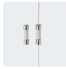
All of the OptiFuse electronic glass and ceramic fuses come with the option of adding an optional axial lead to the ends of the fuse that allow the fuse to be directly soldered into the PCB. A "-P" signifies an axial-lead designation to any standard fuse part number (ex. FSA-P-1A).
